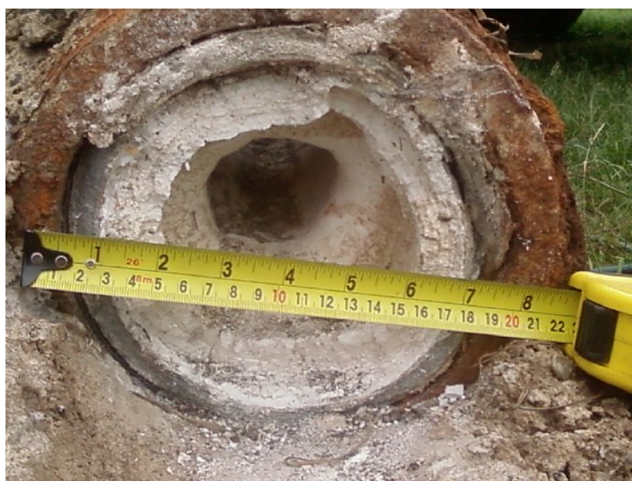
Figure 10.3 Unwanted inorganic scale within water pipework.
